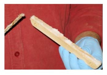
3. Here are the blocks ready to be installed, with holes for the shock cord and rounded corners.
