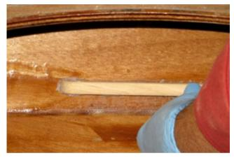
5. As long as the epoxy mixture is thick enough, the blocks will stay in place while the epoxy cures. If you don't think they'll stay put, secure them with masking tape.
