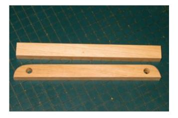
2. Before mixing epoxy, mark the area where the blocks will go and scuff up the surface for a good bond. These blocks will be under quite a bit of load.
