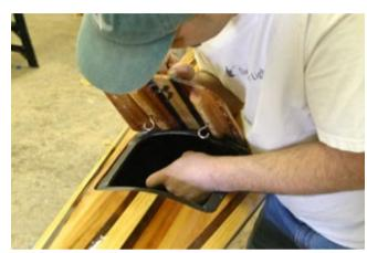
9. You'll need some sort of grab-loop; we put a loop of line through two epoxy reinforced holes in the hatch. As usual, drill oversized holes, fill with thickened epoxy and then drill the correct size.
